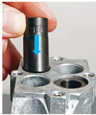
Insert Seat Die in Station #3
