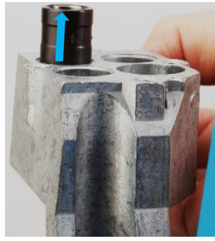
Remove the Seat Die from Station #3
