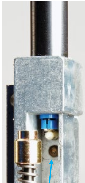
End of Primer Cup Set Screw Stop
