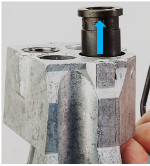
Remove the Size Die from Station #1
