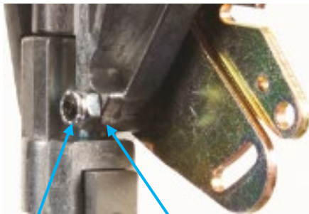
Self-locking Locknut on back of Pivot Screw
