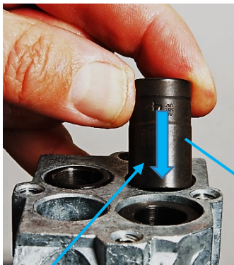
Insert Crimp Die Body #3 here
