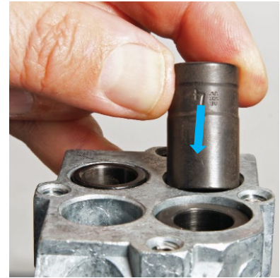
Insert Crimp Die in Station #4
