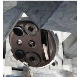
Clean the area under the Shellplate and the Index Ball and Spring
